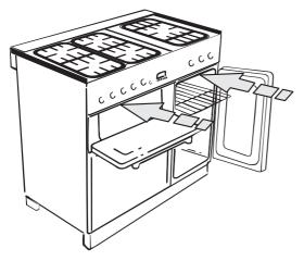
Carefully push the range backwards off the pack base. Remove the pack base tray. Position the range close to its final position leaving just enough space to get behind it.
